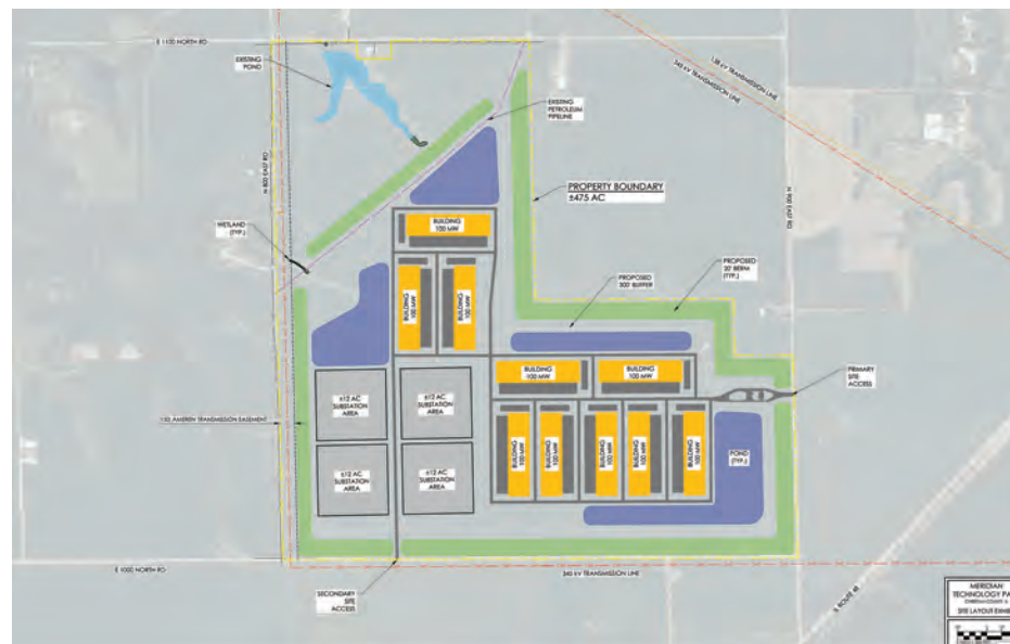
The proposed Eagle Rock Partners' Meridian Technology Park data center would include 10 buildings, each requiring 100 megawatts of electricity to operate. The complex would be in unincorporated Christian County, about two miles southwest of Taylorville, near Illinois Route 48 and at the intersection of East 1000 North Road and North 800 East Road. MAP COURTESY EAGLE ROCK PARTNERS
