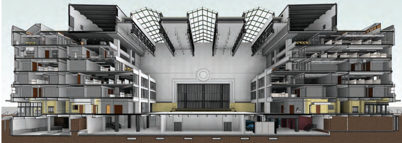
Image shows a section cut view of the completed Armory building improvements. Notable improvements are the new sixth floor, board rooms overlooking the auditorium and historically preserved tiered seating on the fourth floor. CREDIT: COURTESY CAPITAL DEVELOPMENT BOARD
